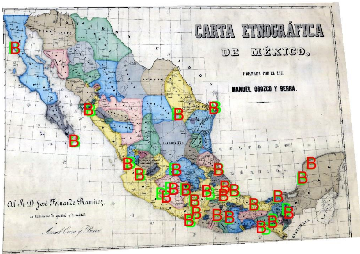
Figure 33 Georeferenced historical map using 2 nd order polynomial transformation along with its control points depicted as the red letter B
